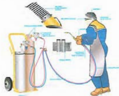
Correct and safe oxygas welding station
