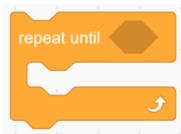
Condition-controlled iteration code inside the block repeats until the condition is met (true)
