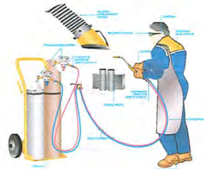
Correct and safe oxygas welding station
