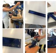
After punching the holes I moved onto the **pillar drill** and created the three holes with a <u>3.2mm</u> bit for the rivets to go in next lesson.
