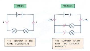
In a series circuit, the potential difference/volt age supplied by the battery is shared by the components.
