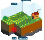
released, it sends out huge amounts of <u>energy</u> causing the Earth's surface to shake violently. The point inside the Earth's crust where the earthquake originates from is known as the <u>focus</u>. The earthquake's energy is released in <u>seismic</u> waves and they spread out from the focus. The <u>epicentre</u> is the point on the Earth's surface directly above the focus. The seismic waves are most powerful at the epicentre.
